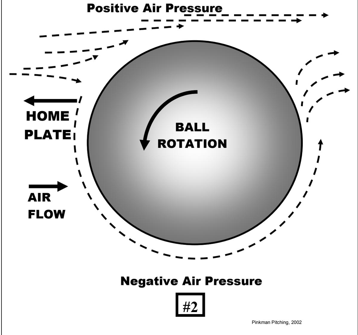
However, unlike an airplane wing, the direction of spin rotation of a ball affects the pressure dynamic. As seen in **Figure 2**, reversing the spin rotation also reverses the air pressures.
